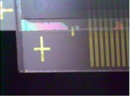
Alignment can be done on the tracks themselves, on special markers (like crosses, thick tracks, round, etc.) on the piece of track that can be seen in between the glass plates, or on special ink markers (see pictures)
