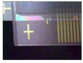
Alignment can be done on the tracks themselves, on special markers (like crosses, thick tracks, round, etc.) on the piece of track that can be seen in between the glass plates, or on special ink markers (see pictures)
