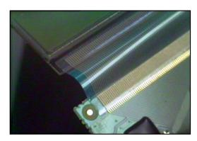
Laptop displays are a good example of ACF Bonding usage. A Chip On Foil technique is used here, one side of the foil is Hot Bar Reflow Soldered to a PCB and the other side is connected using ACF. When using the right produc-Thermal balance in the connecting area is very tion equipment, a extremely reliable joint can be
