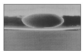
The adhesive normally consists of a mixture of thermoplastic and thermohardening (also known as thermoset- or duroplast-) glues, to get the best of both properties
