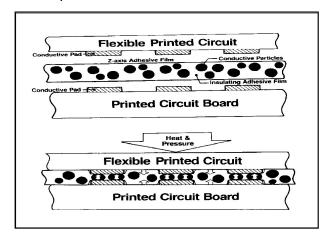
Before connection, an insulating adhesive film separates the conductive particles. When a heating element (normally called thermode) is pressing the top- and bottom circuit board together, with the glue in between, the adhesive will flow, and conductive particles will be trapped, resulting in an electrical connection.
