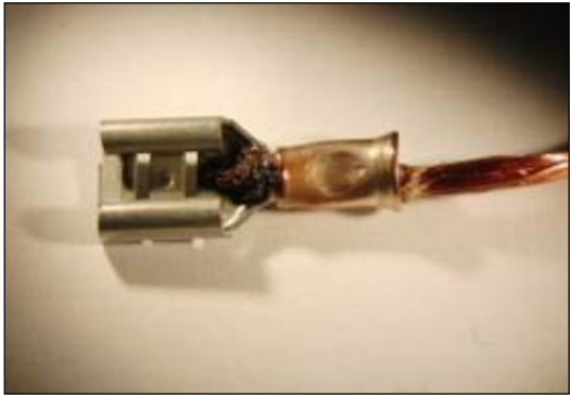
Fig. 12: HF strand on connector.
