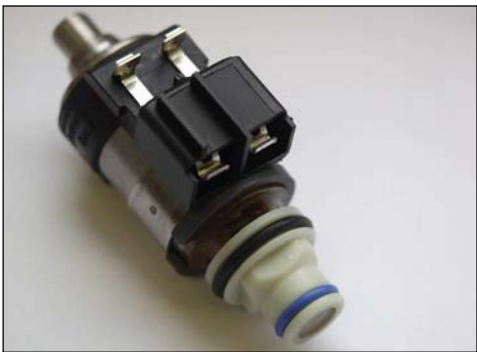
Fig. 11: Lead frame on connector.
